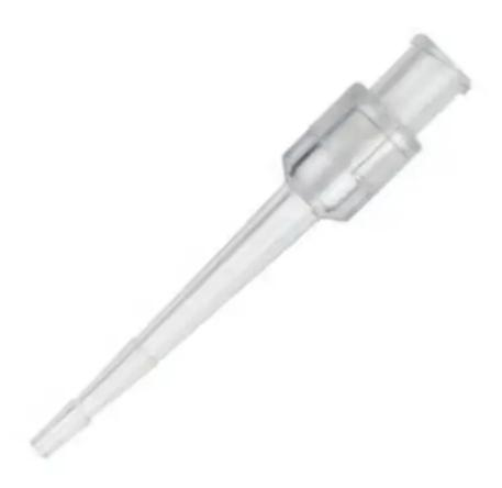
Livanova Vessel Cannulae are intended for antegrade selective vein graft. They are made of a soft PVC tube, with a soft and flexible distal tip, designed to perfuse vessels from 3.0 to 3.6 mm in diameter. They are available in blunt tip configuration, with or without an integral one-way-check silicone valve.
