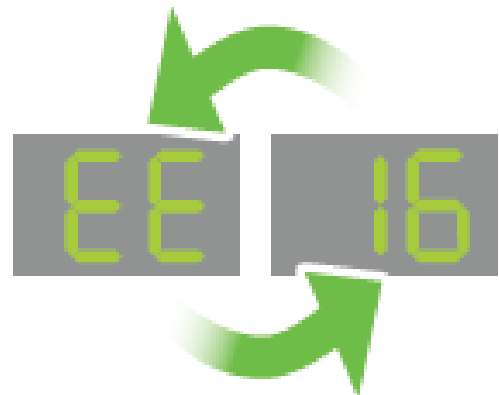
Figure 11: Error codes on the 3T display will flash between error and code number
