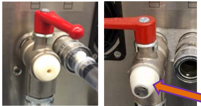
Figure 8: Current Snuffle Valves ( left ) will be replaced with new Snuffle Valves ( right )
