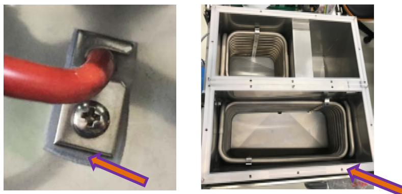
Figure 1: Silicone Gaskets will be added to the Temperature Sensor Mount ( left ) and between the tanks and tank lid ( right )
